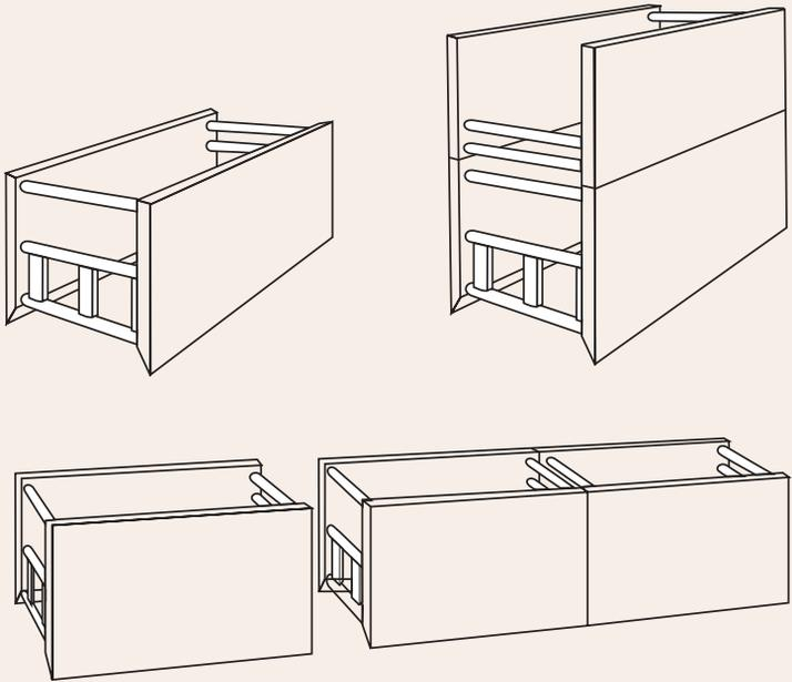
**Figure 2.** *Trench Shields*
