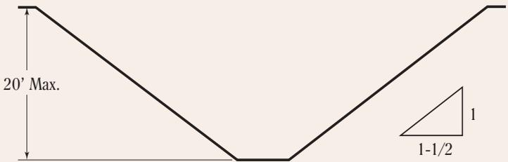
**Figure 1.** Excavations Made in Type C Soil
