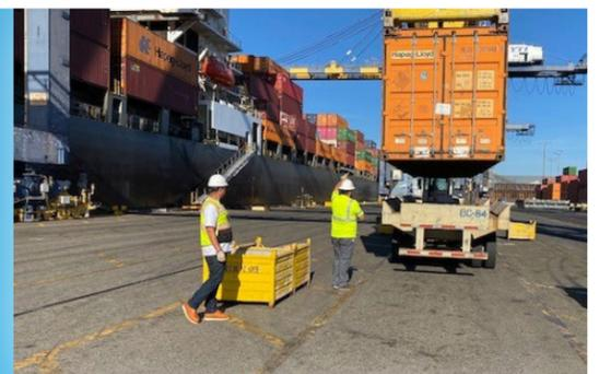
**6** Maintain clear and open radio communication with crane operators.
