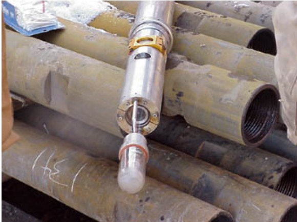
Figure 4. Remote Monitoring Borehole Camera
