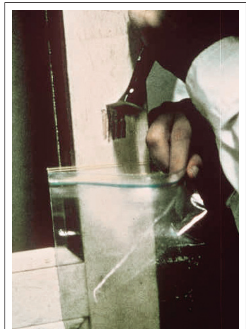
FIGURE 7.5 Removing paint-chip sample.
