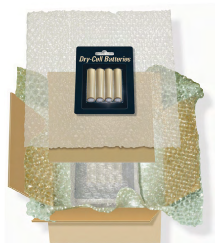
Place batteries and electronic devices containing batteries in a rigid, strong outer packaging
