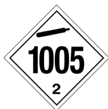
Placard for UN1005, ANHYDROUS AMMONIA SOR/2014-159
