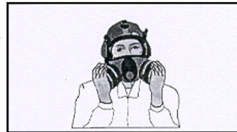
User Seal Check: worker covering inlet and inhaling (negative pressure check)
