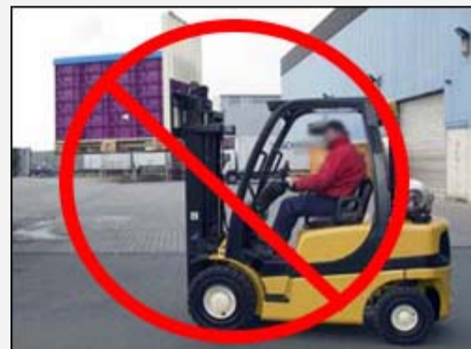
Figure 15. Do not travel with the load elevated.
