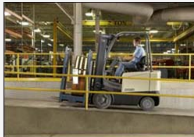
Figure 12. Drive loaded trucks forward going up a ramp.
