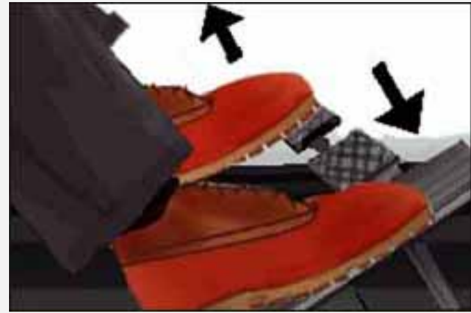
Figure 8. Operator is releasing the inching pedal, setting the direction control to forward and pressing the accelerator. (The brake is the middle pedal.)
