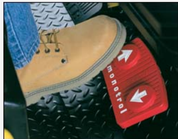
Figure 10. Using pedal to shift from reverse to forward.
