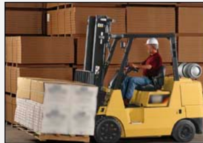
Figure 14. Operator traveling with load lowered.
