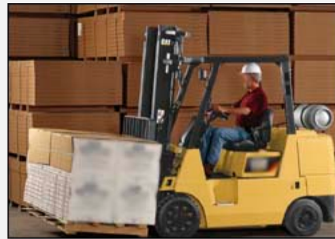
Figure 14. Operator traveling with load lowered.
