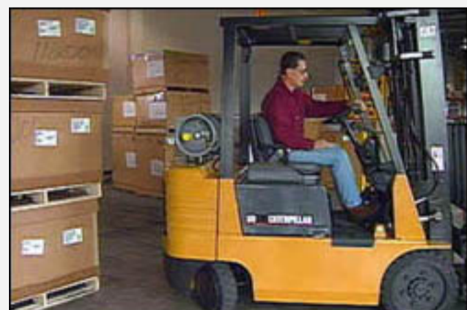
Figure 11. An exaggerated tail swing is caused by rear wheel steering; the operator is turning left and the rear is swinging toward the right.
