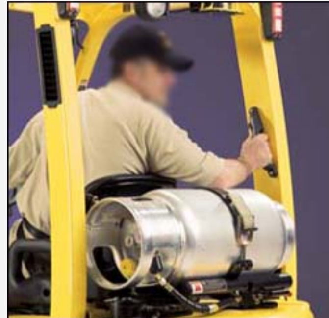
Figure 13. Operator looking in the direction of travel and keeping arms in the confines of the vehicle.
