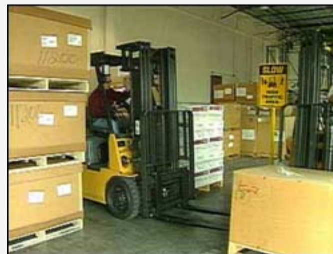
Figure 5. Operator slows down and sounds the horn at cross aisles where vision is obstructed.
