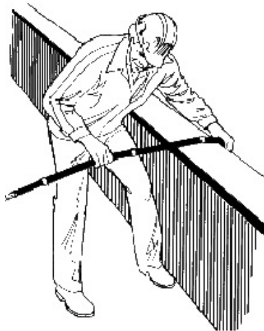
Rubber air hose secured with clamps
